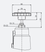
The **Stroke Limiter** is a device that can be installed on all pneumatic angle seat valve. Its function is to influence the plug's position by limiting the stroke of the valve and consequently by adjusting the flow rate. In case of lack of pilot pressure or due to other breakdowns, it acts as a manual emergency override.
