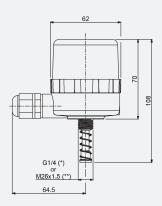
The **Electrical Position Indicator** is an accessory to be assembled on pneumatic angle seat valves series 211/21/211Z3. This device, mounted directly on the valve's actuator, allows to monitor the relative opening and closing status through a local visual control (LEDs) or remotely via electrical signal. It can be supplied individually as an accessory or already preassembled on the valve.
