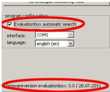
figure 2: Setting of automatic search of the service box and the displayed firmware version after successful initialization.
