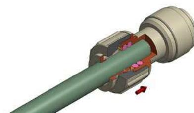
Keep the tube into the fitting completely inserted and screw by hands the nut clockwise up to the fully screwed position. This will grant a perfect seal of the system and the tube will be fully gripped.
