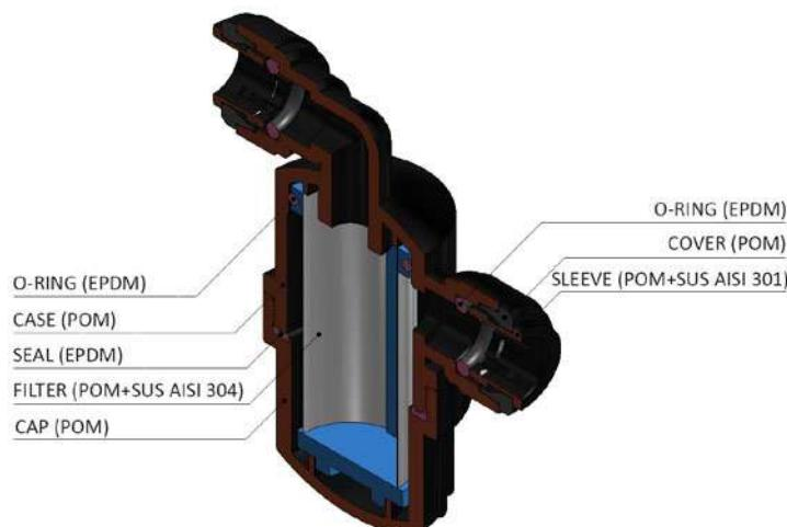
The filter of the Fluidfit range allows to prevent debris with stainless steel filter strainer by 100 mesh in water supply system.
