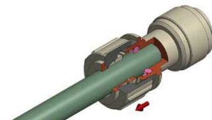
Unscrew anticlockwise the nut by hands making two turns in order to fully release the system.
