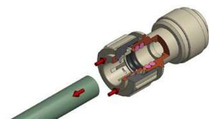
Push the collet in the direction of the body of the fitting and pull the tube keeping the collet pushed in order to disconnect the tube from the fitting.
