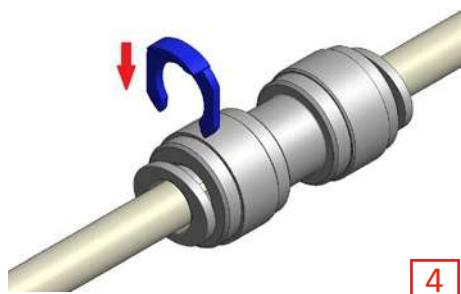
After pulling, insert a locking clip of the right dimension between the fitting body and the collet.
