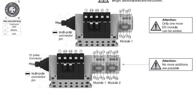
Attention: 2700 solenoid valve manifolds permit up to 22 electrical signals that are not used by manifolds to be made available: these signals can be managed by another manifold and / or by I/O modules.
