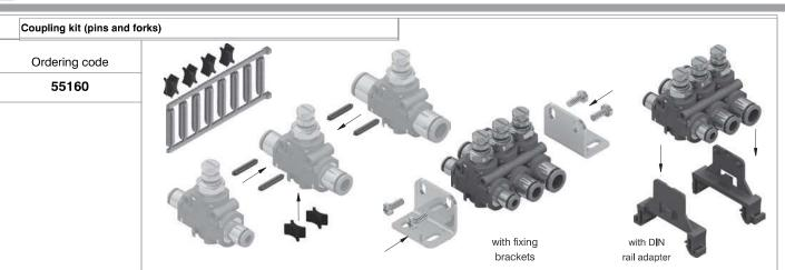
Weight 2,5 gr. - The kit, which includes a series of pins and forks, enables to join together in a fast and safe way the function fittings. The pins, once inserted in the front holes, ensure resistance against forces applied perpendicularly and sideway (for example the insertion of the tube in the cartridges). The forks, once located in the profiled housing ensures that the parts are held together tightly. The kit allows for 5 function fittings to be mounted together.
