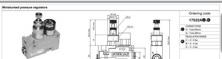
Example: Miniaturised pressure regulators with technopolymer body and integrated gauge, with quick coupling cartridges for tube Ø6 mm and tube Ø4 mm, pressure regulation range 0 - 8 bar Operational characteristic
